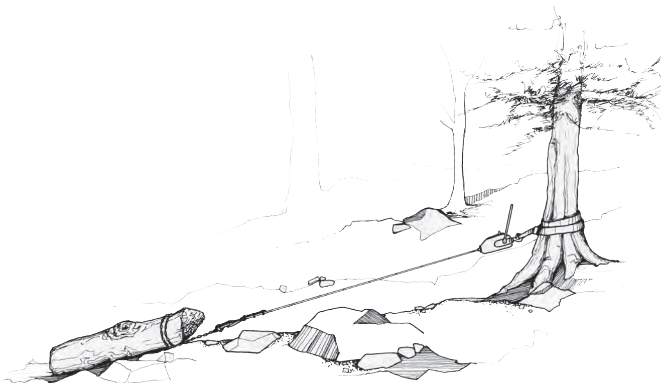
Figure 9–1—A pointed log provides better efficiency in direct-pull ground-skidding.
